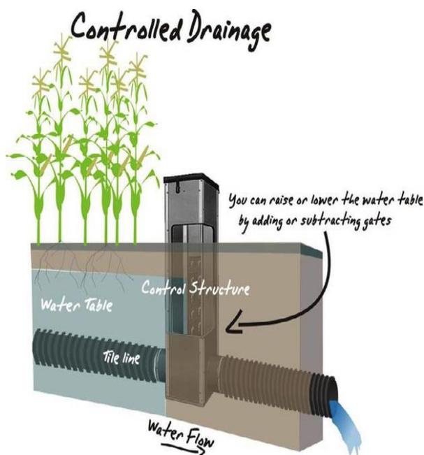
Figure 4: Depiction of a controlled drainage system (Photo credit: [Agricultural Drainage Management Coalition](#))
